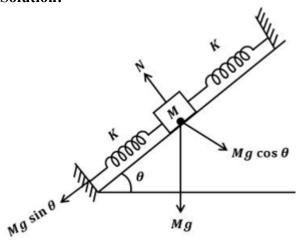
Constant force doesn't change  $\omega$  of the system. (Constant force means force that has constant magnitude and direction. In the direction of oscillation these forces have constant contribution.)
